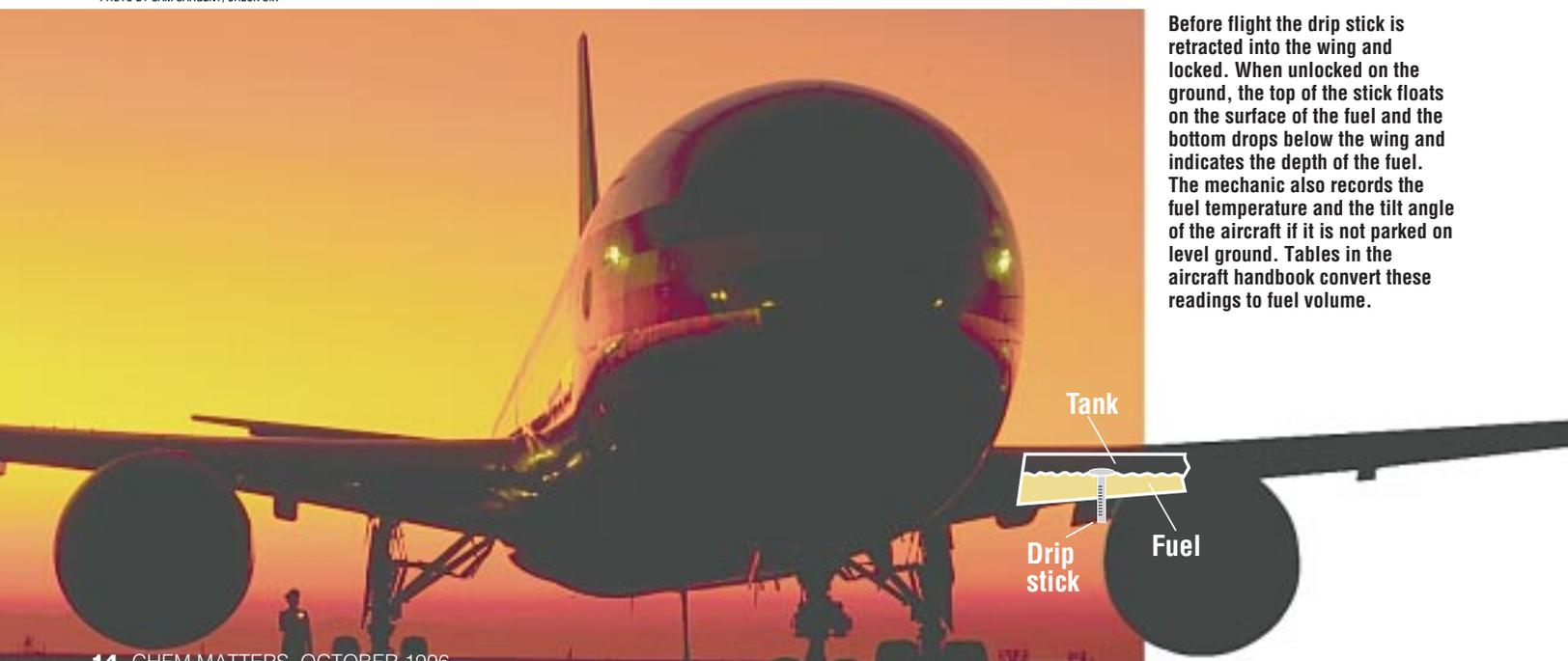
Before flight the drip stick is retracted into the wing and locked. When unlocked on the ground, the top of the stick floats on the surface of the fuel and the bottom drops below the wing and indicates the depth of the fuel. The mechanic also records the fuel temperature and the tilt angle of the aircraft if it is not parked on level ground. Tables in the aircraft handbook convert these readings to fuel volume.
